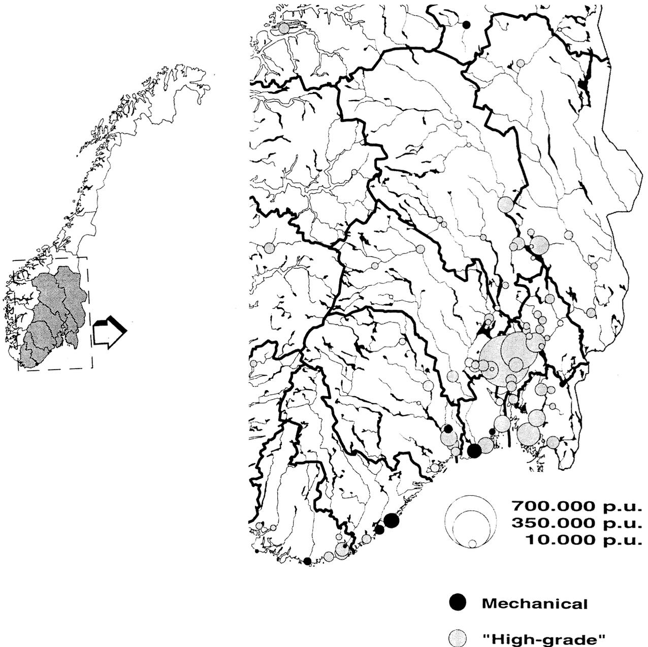
**Figure 3.** Waste water treatment plants in South-Eastern Norway. Location and capacity of mechanical and "high-grade" plants. Plants with a hydraulic capacity of 5000 p.u. or more in 1991
